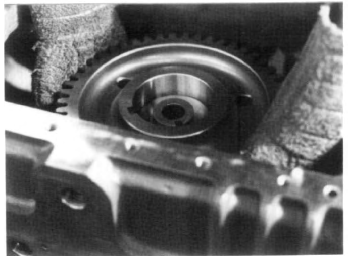
FIG. 6.1-4 Using heat protective gloves take large gear from heater, orient keyway suitably and lower onto intermediate shaft. Be sure gear is fully on shaft.
