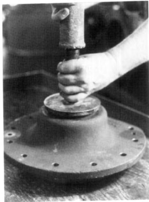
FIG. 6.4-14 Seat oil seal in speed carrier.
