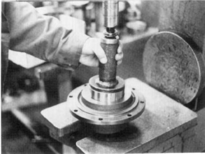
FIG. 6.7-1 Press bearing cups into carrier with suitable press.
