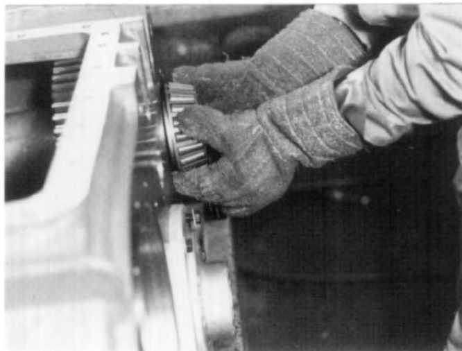
FIG. 6.2-3 Still wearing gloves quickly assemble bearing cone to rear of upper shaft.
