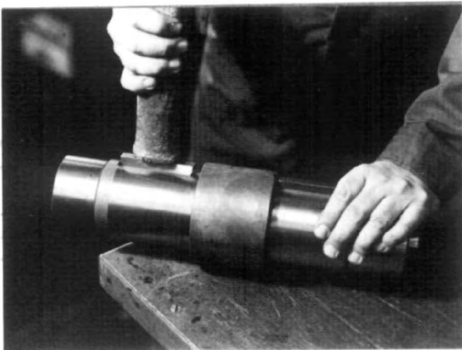
FIG. 6.1-2 While gears are warming, assemble keys into keyways in intermediate shaft. These should be a light drive fit and a soft brass drift may be used.
