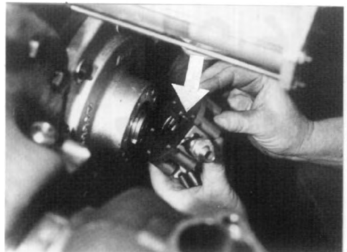
FIG. 6.8-4 Assemble pump end cap with 2 cap screws, just started, to carrier. NOTE - Be sure pin (arrow) on flat mating face of cap engages shoulder slot on end of pump. Turn pump assembly if necessary to place cap in correct orientation for plumbing.
