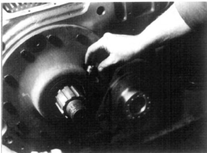
FIG. 6.4-18 Grease bore of speedo adapter and slide over pinion, screw into carrier, tighten to appropriate torque.
